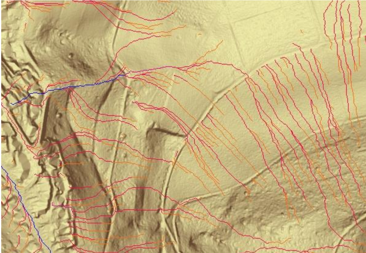
Figure 30: Unweighted flow accumulation map of Ittmecke. There is a residential area to the far left. The lines are accumulation flow lines from 500 cells up (orange). Red lines start at 1000 cells and blue lines at 10.000. The blue line in the lower left corner runs atop roads. It is not critical with regard to erosion. This shows that the unweighted flow accumulation map can only be used to understand the general situation.
