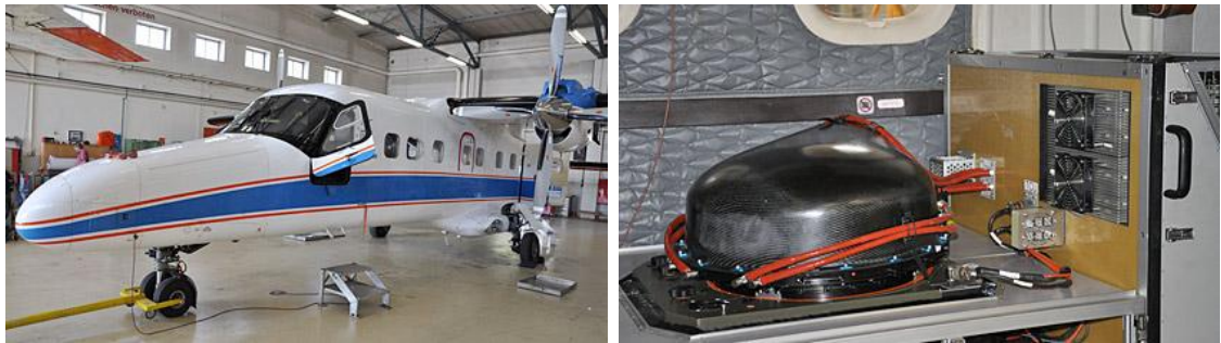
Figure 5: Picture of the Dornier DO-228 on which the sensor was installed, and the APEX sensor (Images from RSL, University of Zurich)
