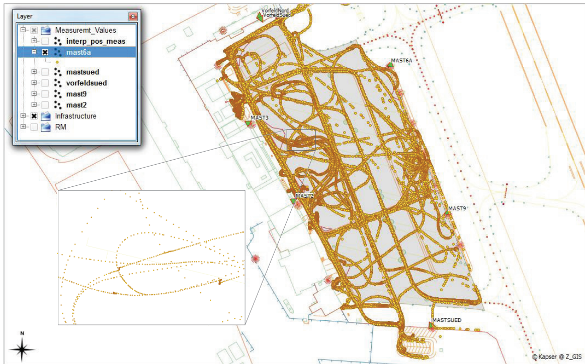
Figure 3.12.: Spatial WLAN measurements to AP mast6a at main apron of Salzburg Airport
