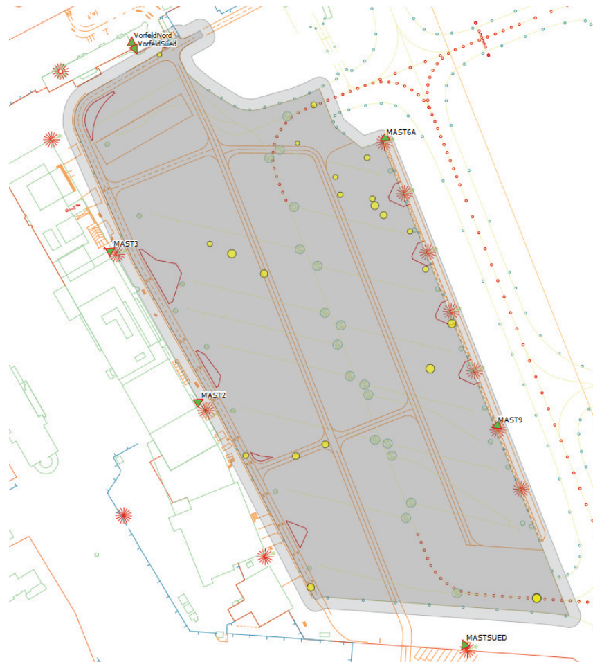
Figure 3.19.: Final measurement reference value distribution for AP mast 6A
