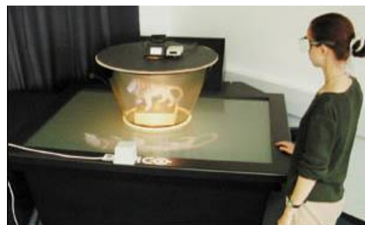
Abb. 26: Optical-see-through Display (Quelle: www.cgw.com )
