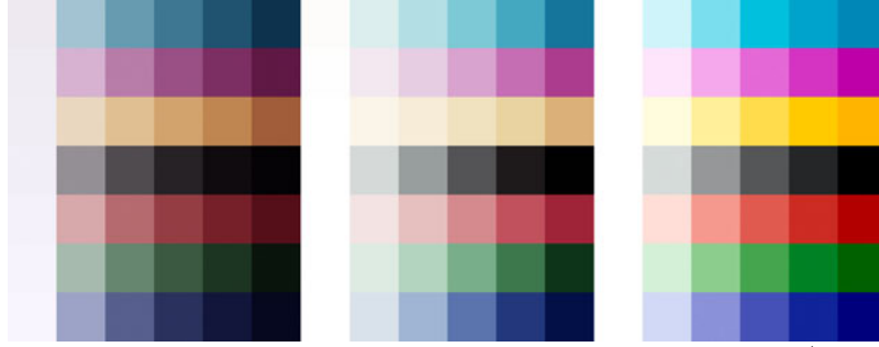
Figure 4.7: Spline interpolation of white to black color patches for UCL (aperture F8). The left image shows the original image coming from the camera, the center image shows the result after applying the spline correction and the right color target shows the referenced used for creating the spline
