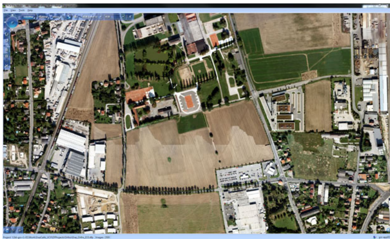
Figure 2.1: Sample for radiometric sensor fusion problem in Graz, Austria. The color shift is visible in the center of this screenshot in the field.
