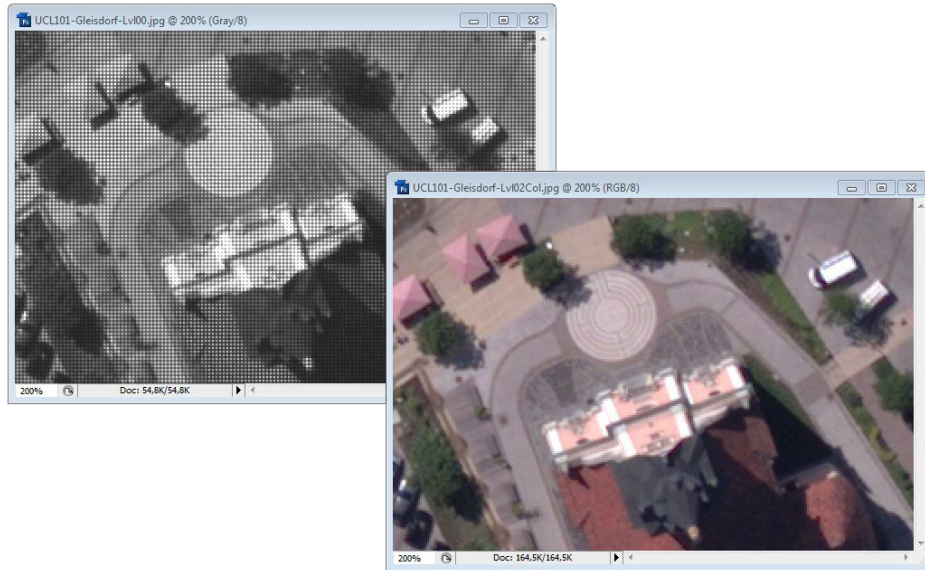
Figure 2.5: Raw Bayerpattern image (back left image) and final demosaicked image (front right image)
