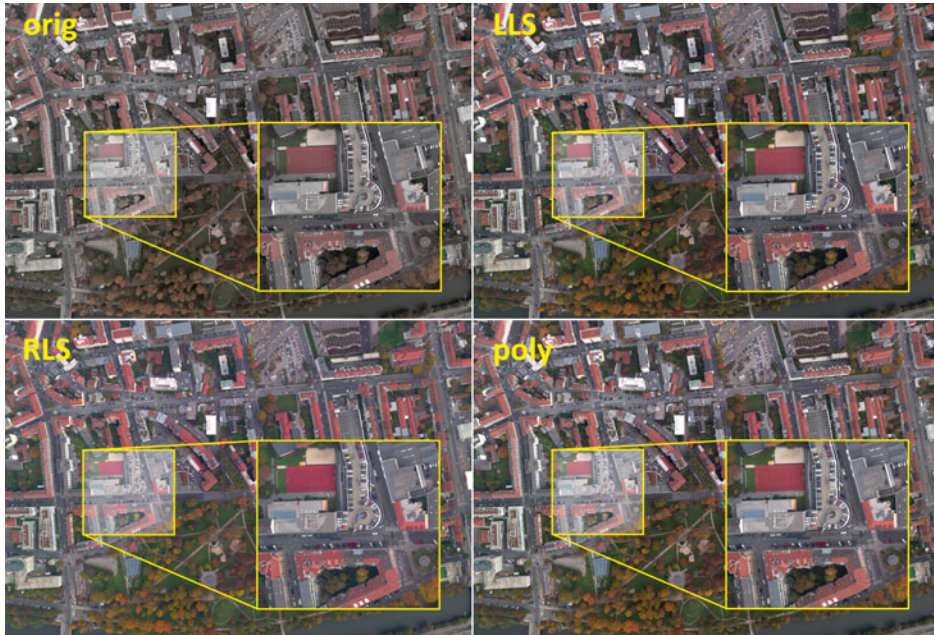
Figure 6.3: Comparison of aerial images (from UCL) in an urban area in Graz, Austria, treated with the three different color correction methods in the following order: upper left: original UCL image, upper right: LLS corrected image, lower left: RLS corrected image and lower right: polynomial adjusted image
