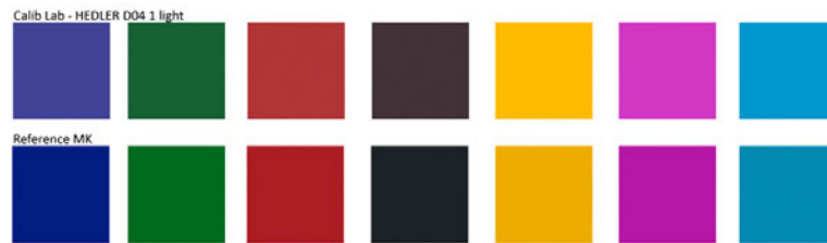
Figure 4.6: Available reference information (top: verification with spectrometer, bottom: original reference data from Kodak IT8 target)
