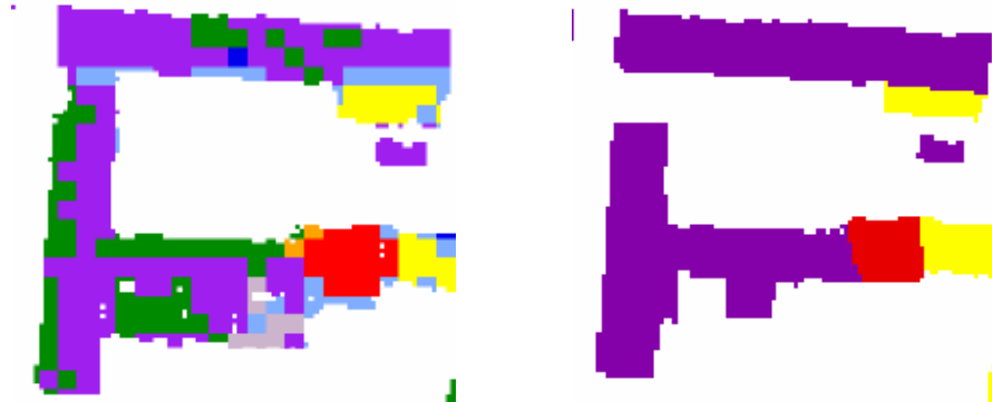
a) Slate roof (purple) with many clusters of wrongly classified bitumen pixels (green). SVM classification left, reference right
