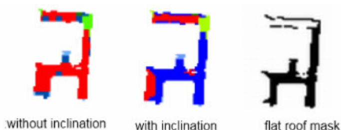
Tile roof, mostly correctly classified without inclination, is classified as stone slab in those parts that are labelled "flat" in the inclination mask
