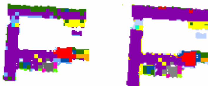
Improvement of the classification of slate (purple) by the incorporation of inclination information. Left, SAM without inclination, right SAM with inclination
