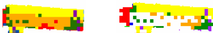
b) Detail of SAM classification with an angle of 0.5 rad (left) and an angle of 0.1 rad (right). Even when the angle is very small, pixels are already classified as copper (orange) instead of aluminium (yellow).
