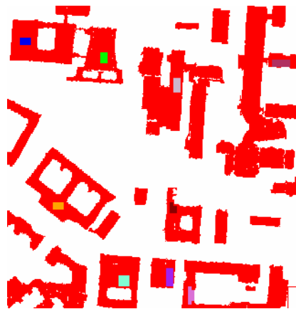
Figure 35: Example of overfitting of the training data. Detail of the SVM classification with the parameter pair: \gamma = 2^{-40} , C = 1000 . The training data (displayed in different colours) are correctly classified, the rest of the pixels are assigned to one class only (red colour)
