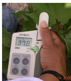
Figure 4.9: Minolta's SPAD-502 Source: BRONSON 2005
