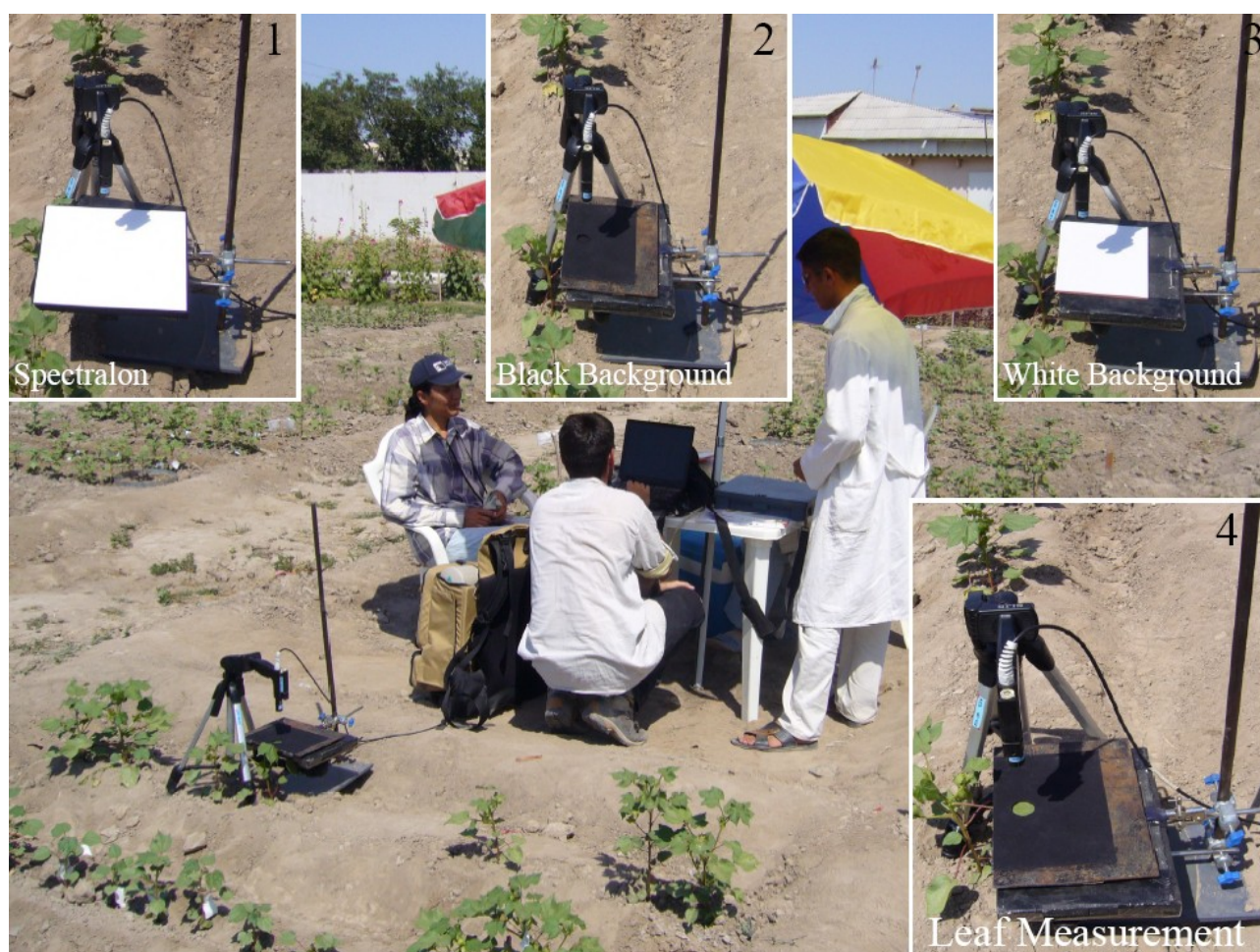
Figure 4.12: Reflectance Measurement Procedure at Leaf Scale
