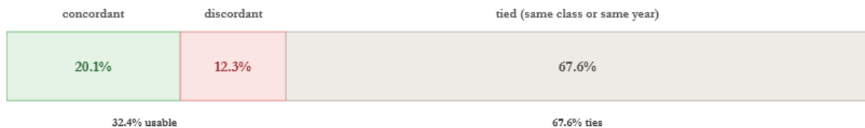
Figure 21: The share of concordant, discordant and tied pairs, shown here by the example of moisture level vs time of attack. The large share of tied pairs is better handled by Kendall than spearman
