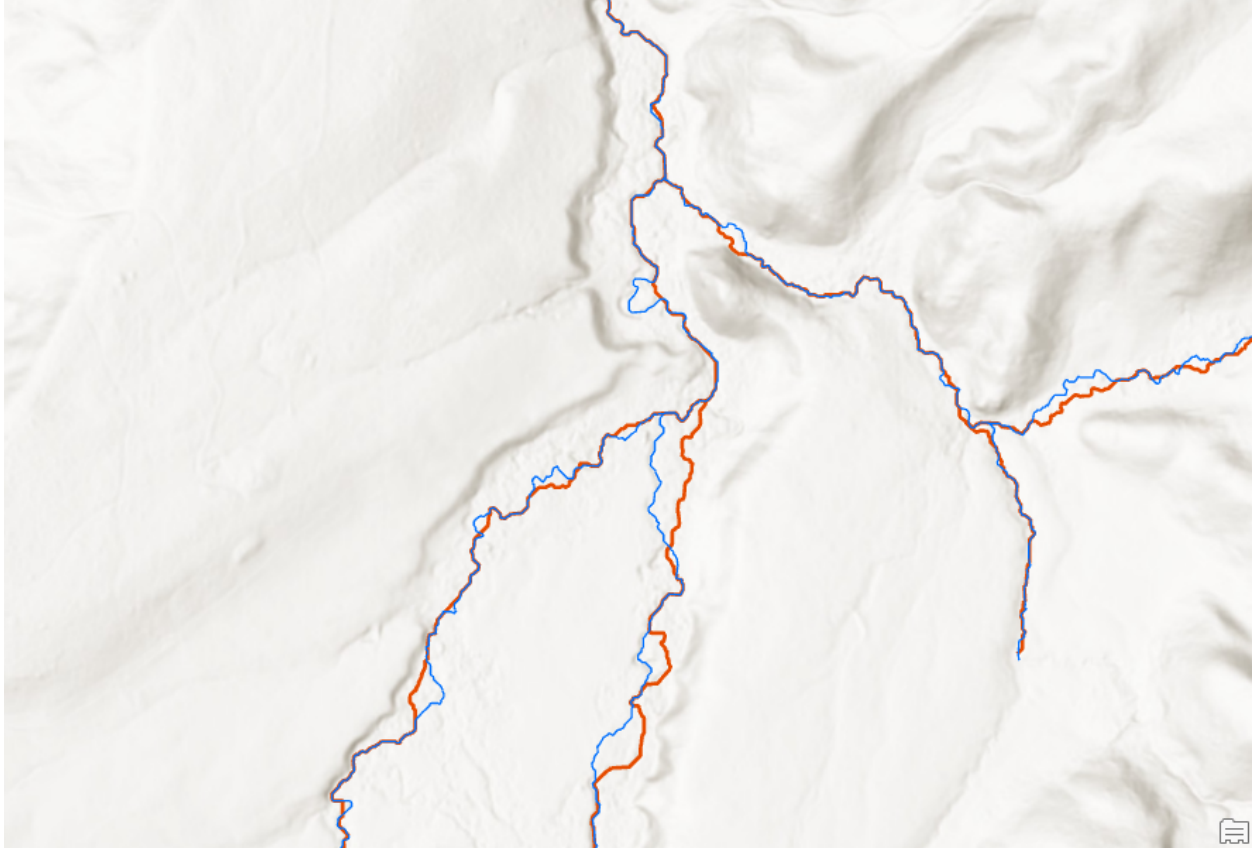
Figure 9 - Example of misalignment between DEM derived, hydrologically correct segments (blue) and segments containing data from BRAT (red). After completing the steps outlined above, the PotentialDamPerKm values from BRAT were transferred to the closest point in the DEM-derived dataset and then summarized for the 300 m segments that were generated for streams in the DEM-derived dataset
