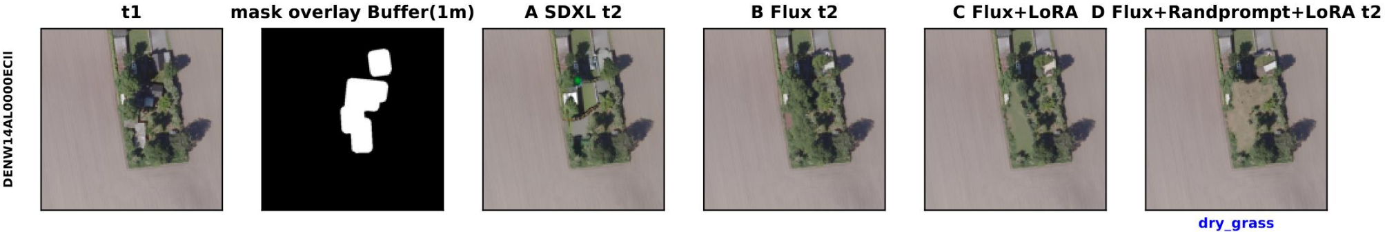
Figure 4 Qualitative comparison of synthetic change generation in Experiment 1. The vertical labels on the left indicate the ALKIS ID as a spatial reference. Original T1; target area mask; SDXL (E1-A) with illogical structures; Flux (E1-B) with extremely vivid textures; Flux + LoRA (E1-C) with realistic but monotonous results; Flux + random prompts/LoRAs (E1-D) with both realism and diversity. The labels under column indicate the specific target class (e.g., “gardens,” “agriculture fields”).
