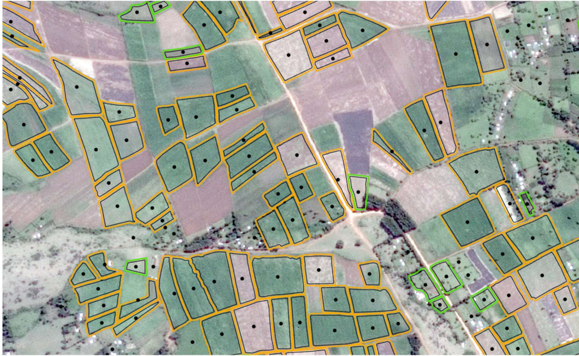
Figure 2.15 - Example of centroid generation following the application of a 5m negative buffer to sugarcane and non-sugarcane training polygons.
