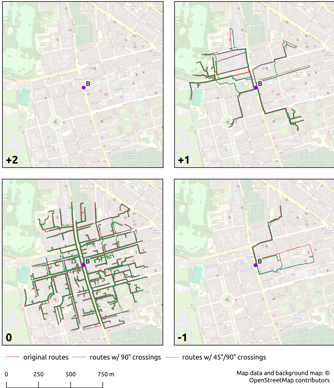
Figure 4.7: Map of resulting routes for start point B grouped by a45 type crossing count differences
