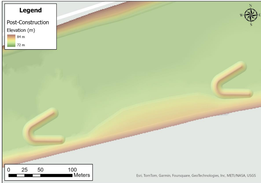
Figure 21 Digital terrain model of the river Drava in the post-construction state – detail around river kilometre 6 showing chevrons 5D-3 and 6D-1
