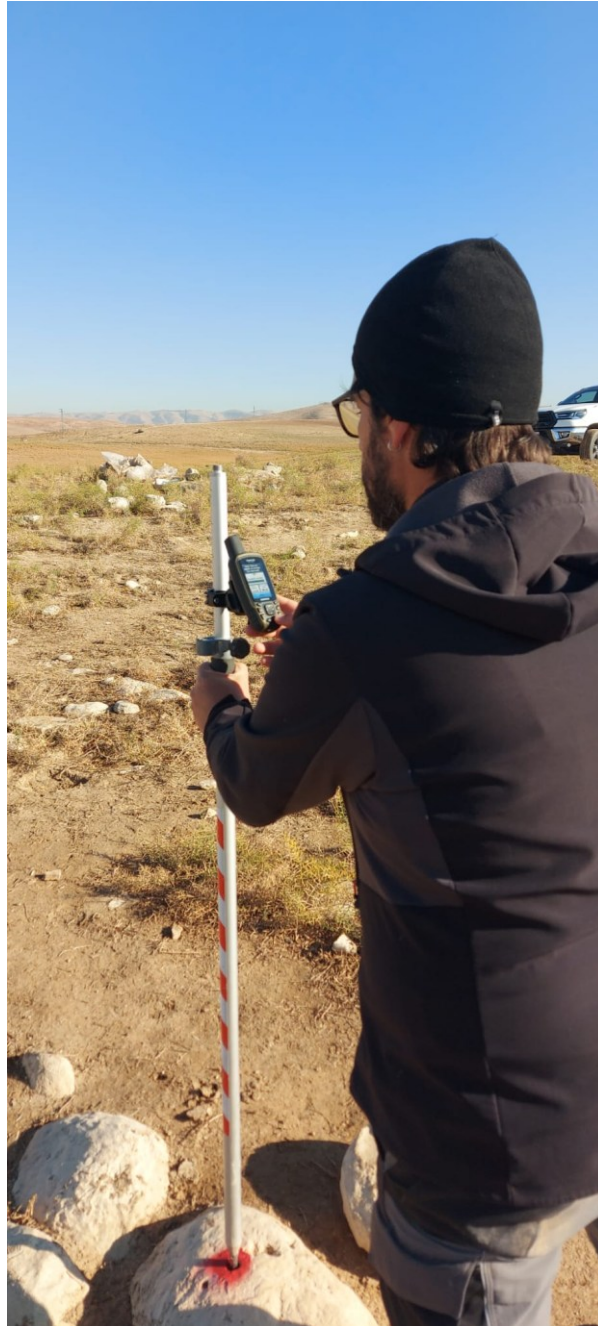
Figure 2.5. Control-point measurement with the consumer-grade GPS receiver on a levelling pole (©ReLand).
