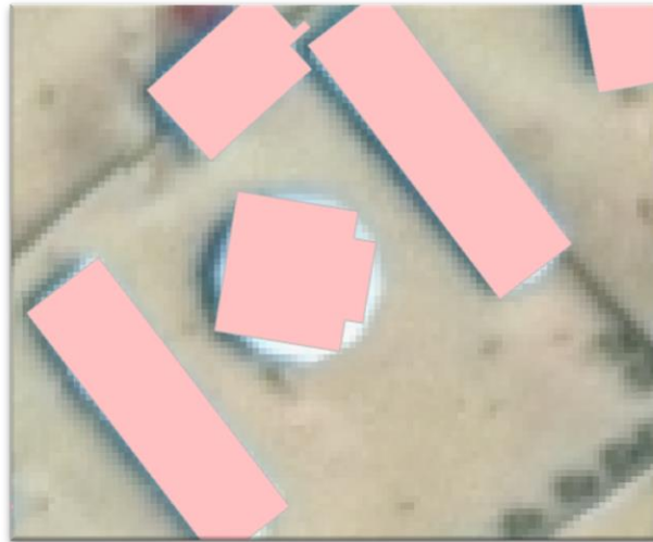
Figure 48: Wrong method for round Facility Buildings
