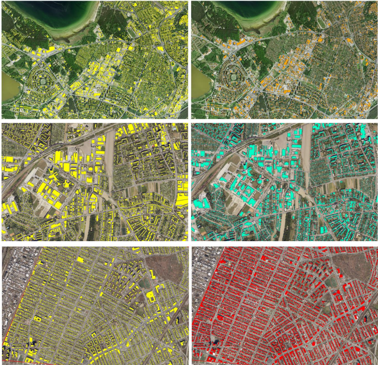
Figure 35: Successful building extraction examples. FT USA VNA on the Tallinn target area is shown on the top (orange), FT USA TLN on the Vienna target area is shown in the middle (turquoise), PT USA on the New York II target area is shown on the bottom (red). Ground reference (yellow) is depicted on the left. Appendix 6 provides the images at a larger scale.
