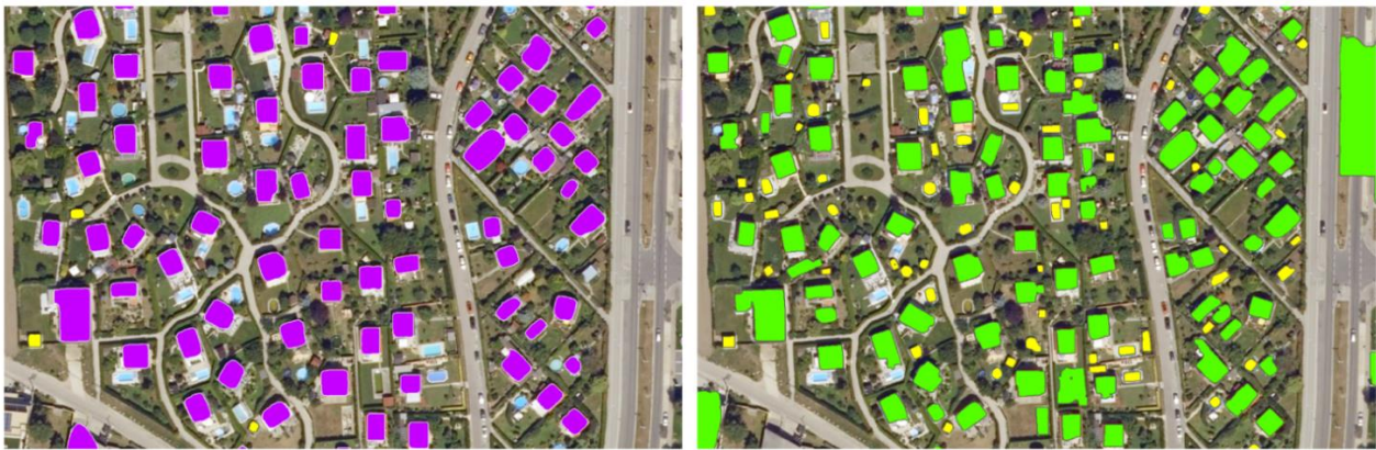
Figure 20: Building extraction results the Vienna target area. PT AFR (purple) and FT AFR VNA (green) on the right after the deletion of small objects. The erased small objects are highlighted in yellow.
