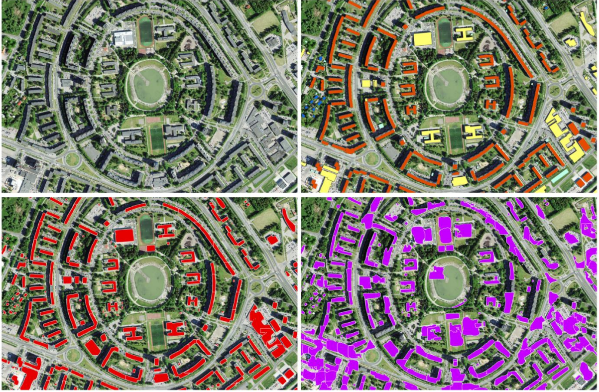
Figure 12: Building extraction results on the Tallinn target area. The top row shows the satellite image (left) and the ground reference (right). The bottom row depicts the extraction result of PT USA (red) and PT AFR (purple).
