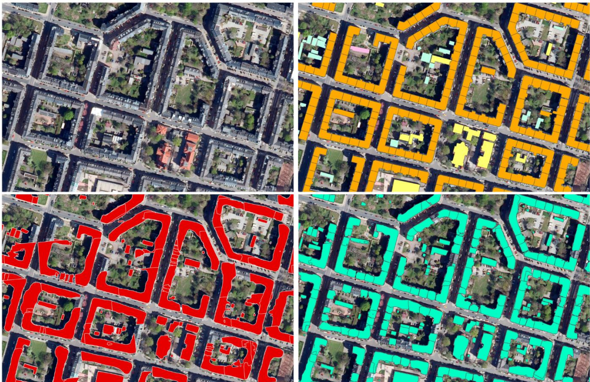
Figure 15: Building extraction results on the Chemnitz target area. PT USA (red) and FT USA TLN (turquoise). The top row provides the ground reference.
