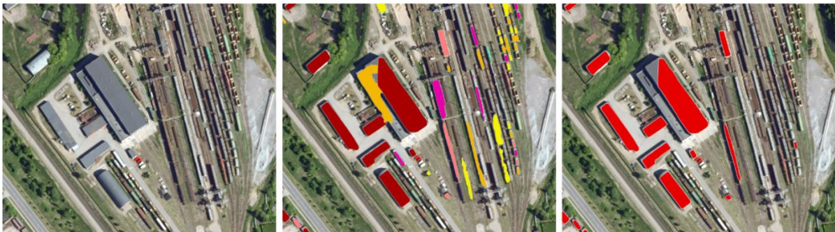
Figure 24: Building extraction results on the Daugavpils target area. PT USA (red). The satellite image of the Daugavpils industrial train station is depicted on the left. The extraction confidence of PT USA is depicted in the middle with the same colour code as above.
