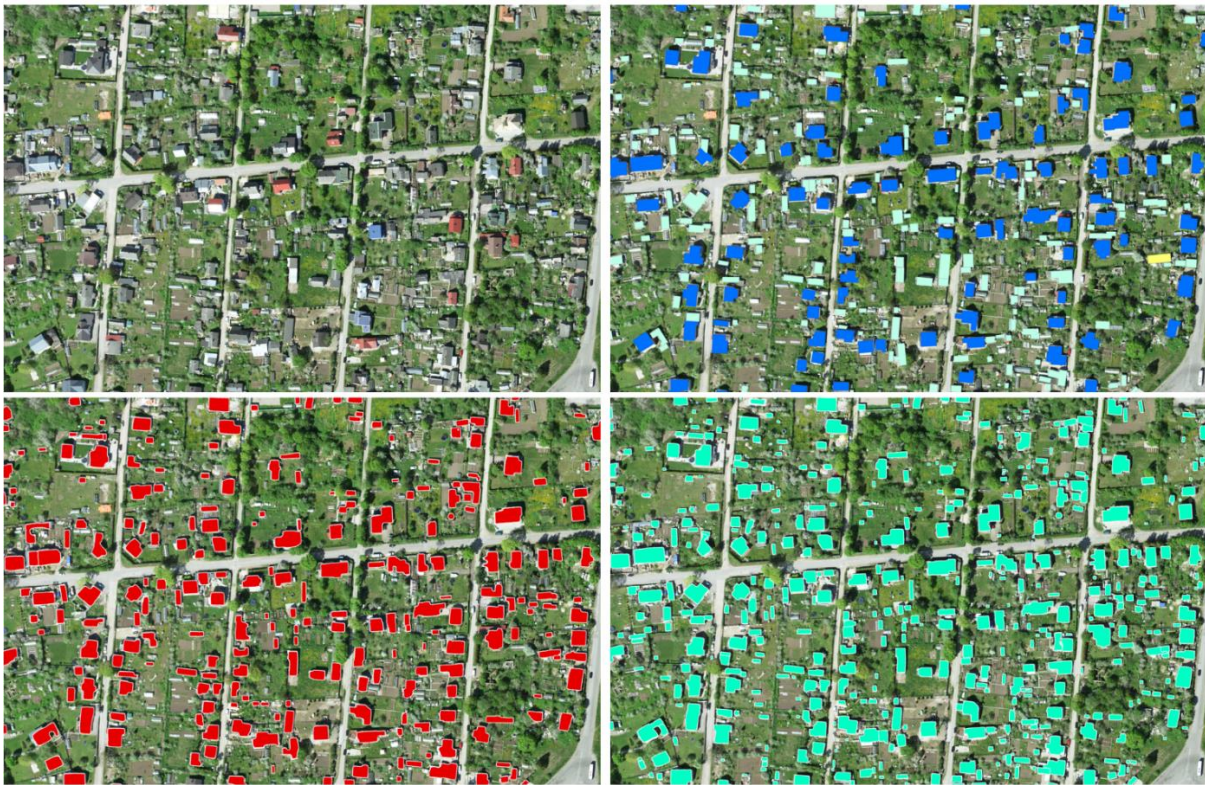
Figure 16: Building extraction on the Narva target area. PT USA (red) and FT USA TLN (turquoise). The top row provides the ground reference.
