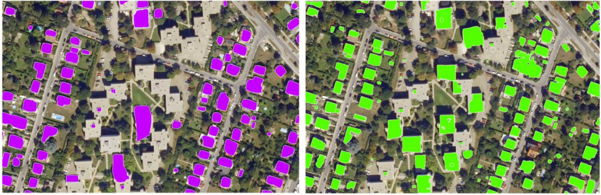
Figure 14: Building extraction results on the Vienna target area. PT AFR (purple) and FT AFR VNA (green). Both models extract the single family houses well. PT AFR fails to extract the apartment blocks in the middle.
