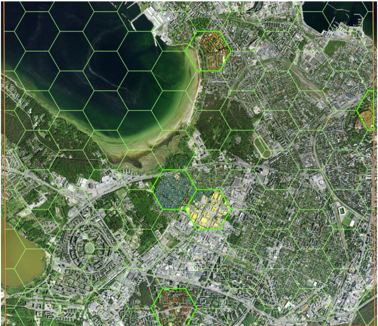
Figure 9: Subdivision of the Tallinn target area with the tessellation grid (green). The reference building labels of the selected micro-regions are displayed.
