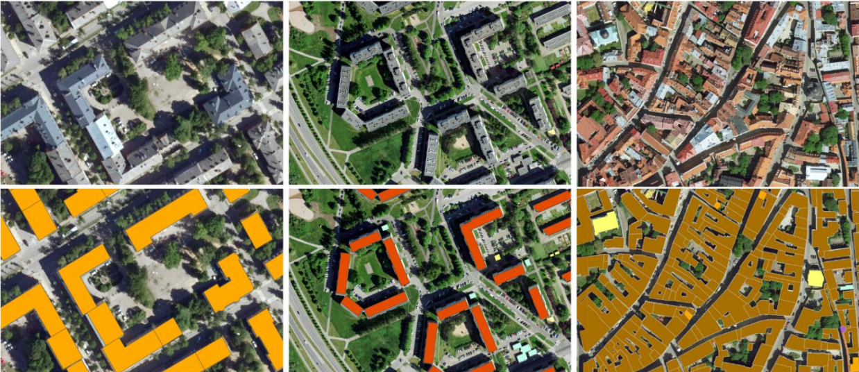
Figure 7: Building type categorization. Apartment buildings (orange) have various roof types, apartment blocks (red) are usually separated and have a flat rooftop. Historical districts (brown) can be found in the Tallinn and Kosice target areas. [From left to right].
