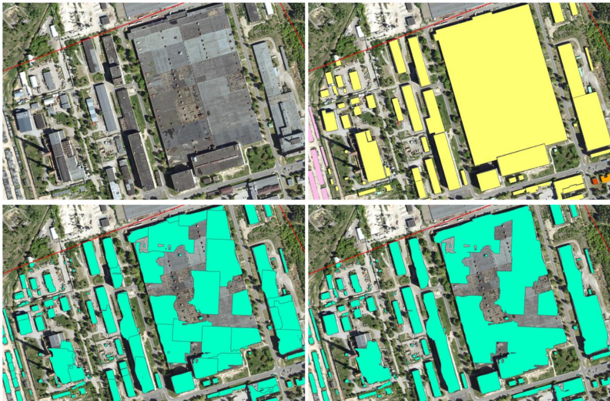
Figure 17: Building extraction on the Daugavpils target area. FT USA TLN (turquoise) on industrial buildings. On the bottom left, the extraction result is depicted without post-processing. On the bottom right, the result after the dissolve boundaries post-processing is depicted. The top row provides the ground reference.
