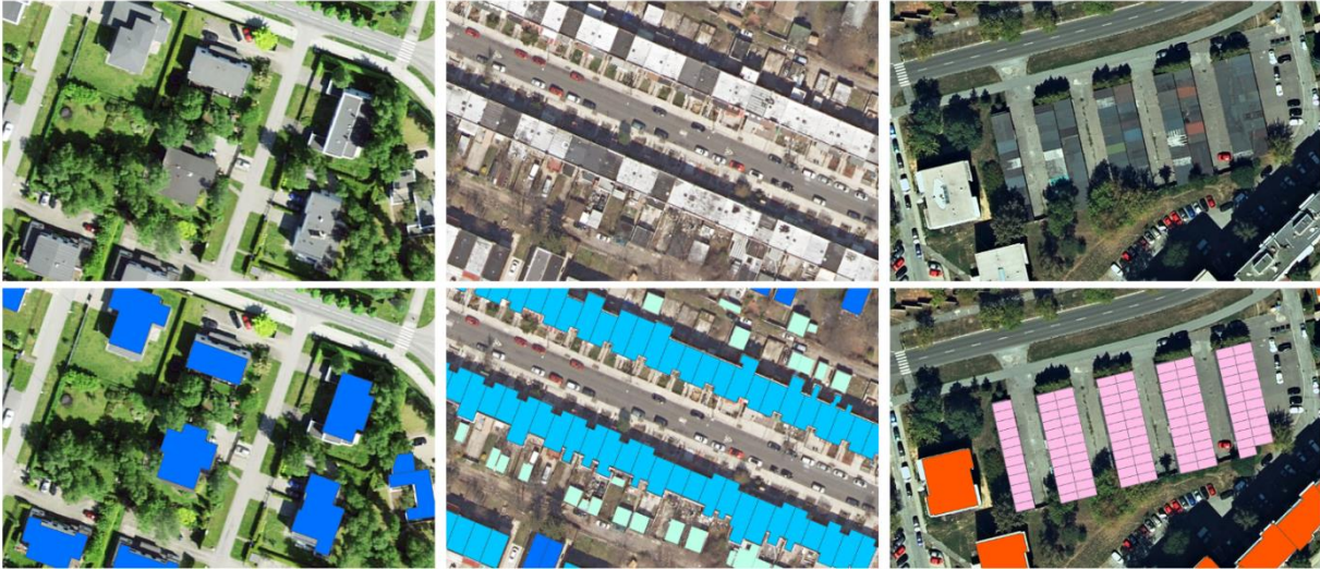
Figure 6: Building type categorization. Single house family buildings (dark blue), terraced houses (light blue), garage blocks (pink). [From left to right].
