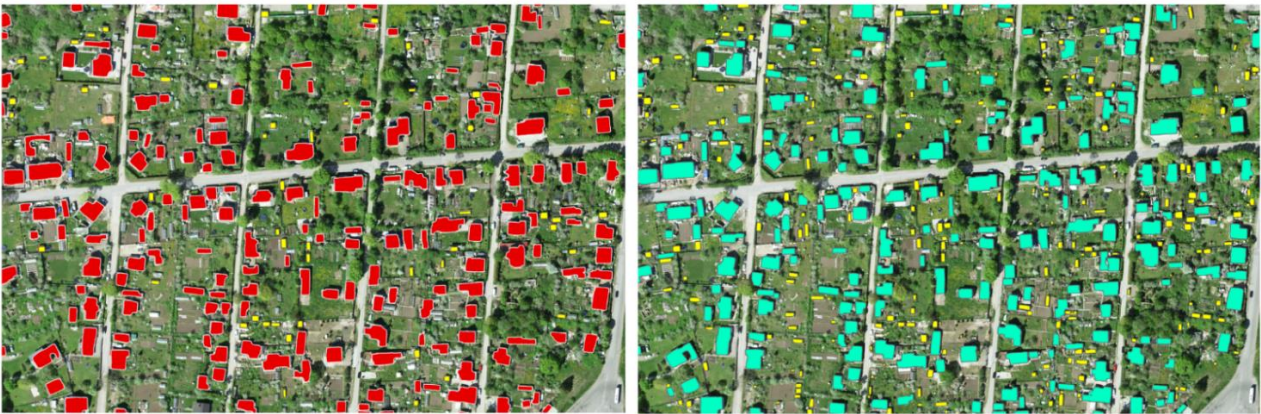
Figure 19: Building extraction results on the Narva target area. PT USA (red) and FT USA TLN (turquoise) on the right after the deletion of small objects. The erased small objects are highlighted in yellow.
