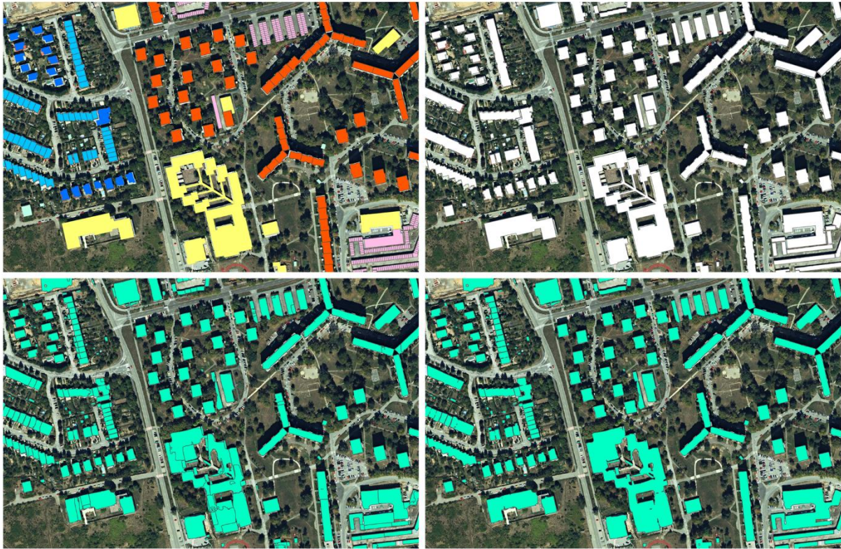
Figure 18: Building extraction on the Kosice target area. FT USA TLN (turquoise). On the left before the post-processing and on the right after the execution of the dissolve boundaries step. The top row provides the ground reference, Ground reference after the application of the dissolve boundaries post-processing is shown on the right.
