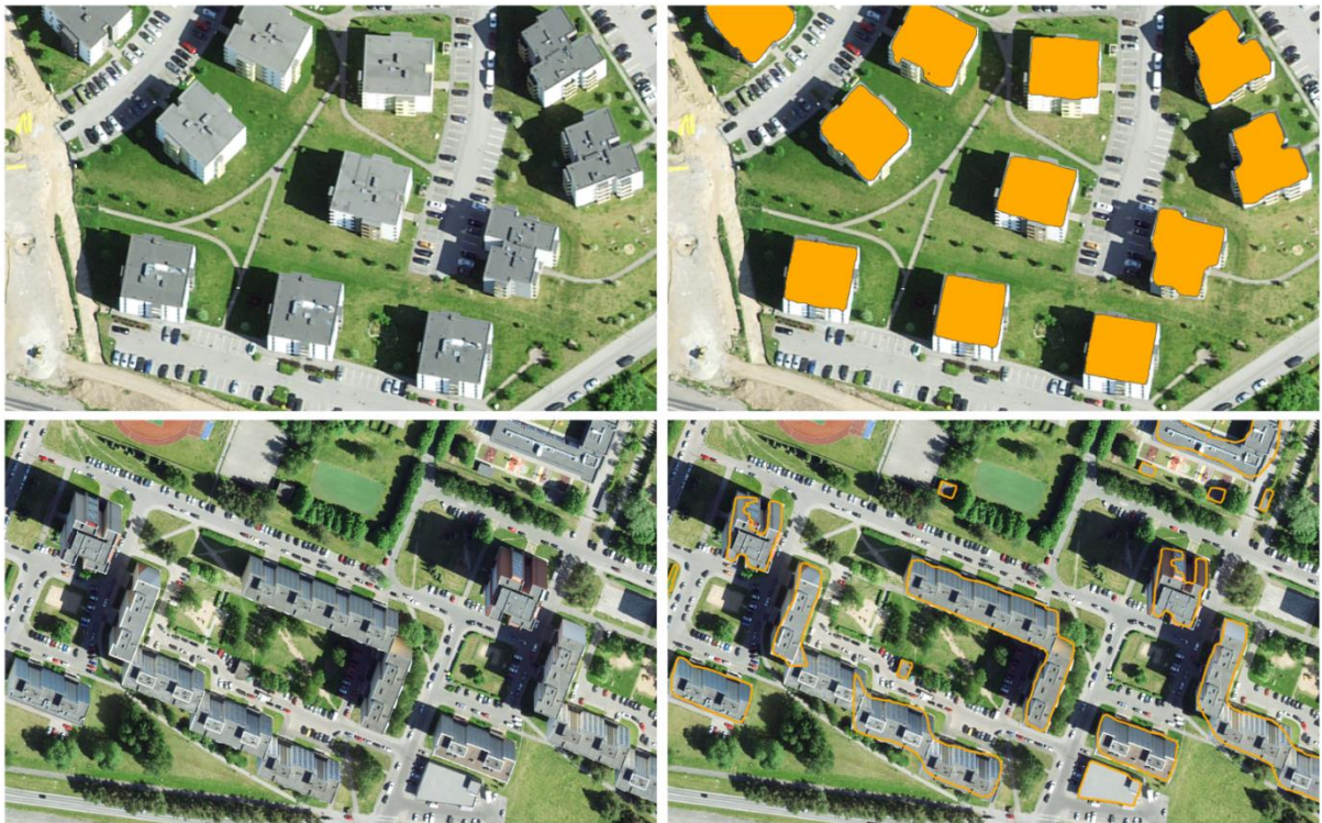
Figure 1: Off-nadir impact on building extraction. Successful building extraction on low off-nadir image is shown on the top. The negative effect of a large off-nadir is shown on the bottom.
