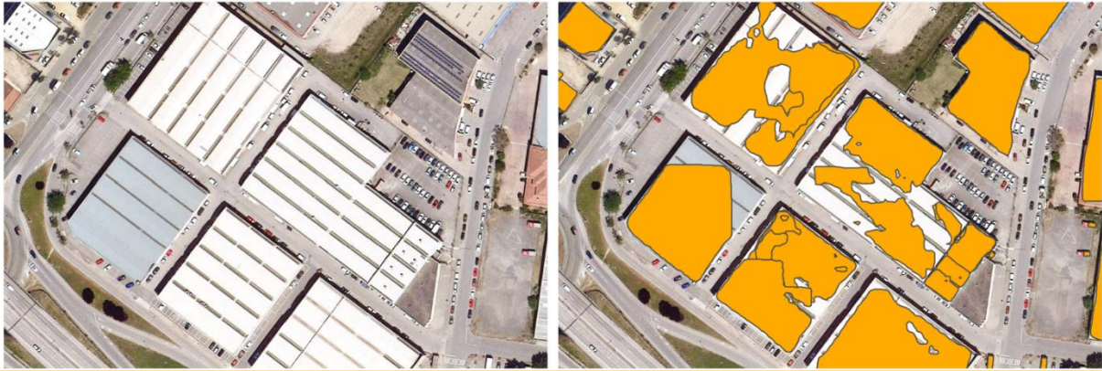
Figure 9: Building extraction on large objects and complex roof structures. Mask R-CNN models often generate multiple predictions for the very same object (in orange).
