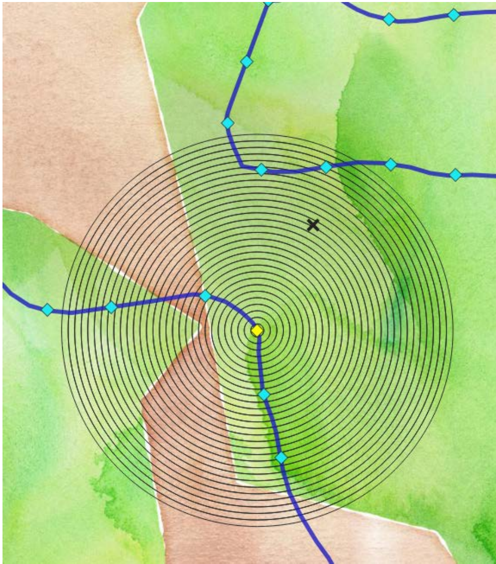
Figure 15 – With one stop position point as centre (yellow diamond), 50 buffer rings are calculated (for better visibility, the graphic only contains 30 rings). Each ring represents 10 seconds of travel time by foot. The diameter of the ring spatially intersecting the accident site (black x) corresponds to the walking time needed. 23
