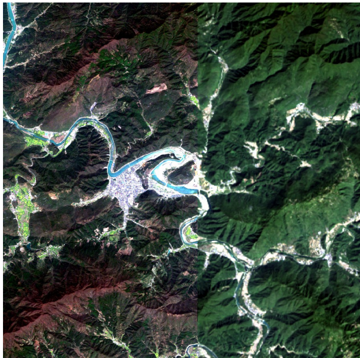
Figure 9: Differences in resolution between the RapidEye image (left) and the Landsat 8 image (right)
