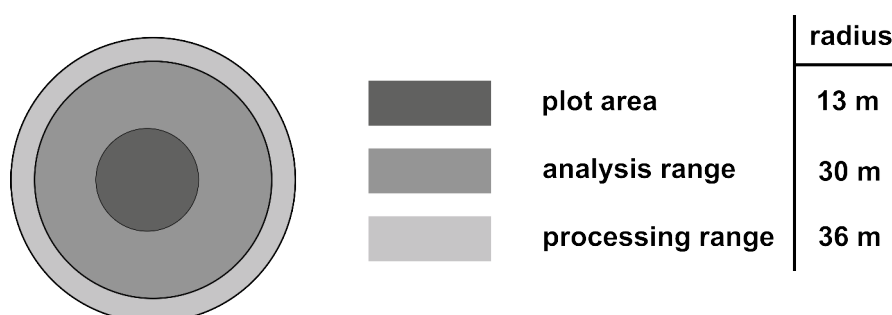
Figure 2.4.1: Analysis and processing ranges around a plot
