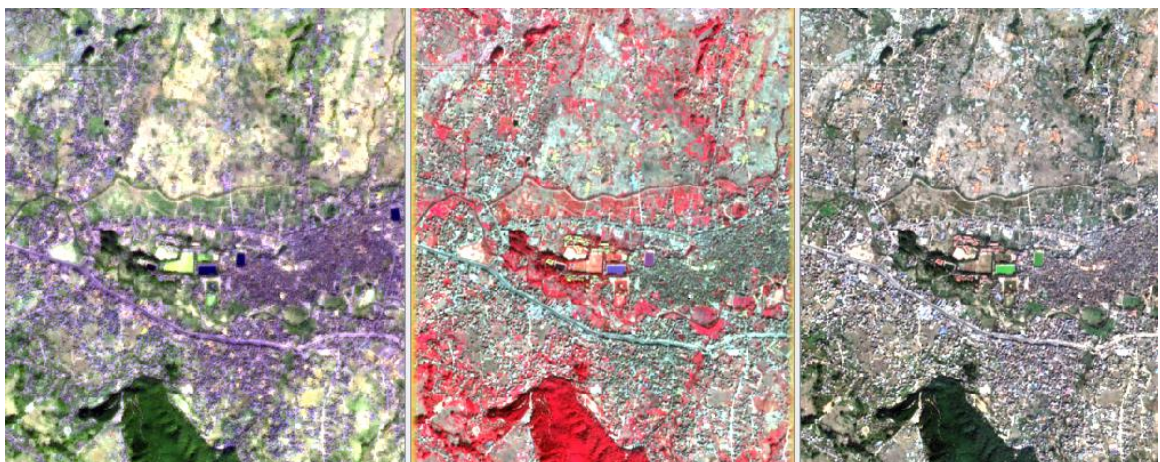
Figure 2. 7: Band composites of S-2 image – false color urban (left), false color infrared (middle), natural color (right)
