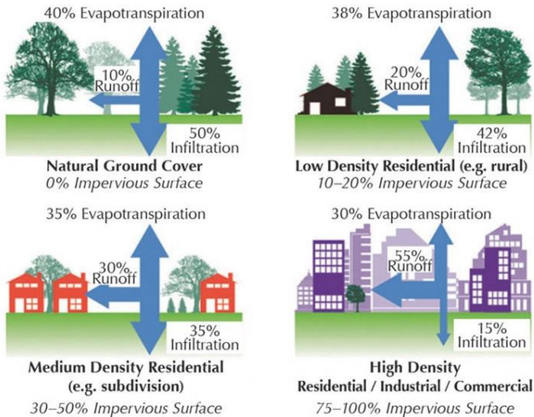
Picture 4: Infiltration effects on impervious surface (John Hopkins University, 2020)
