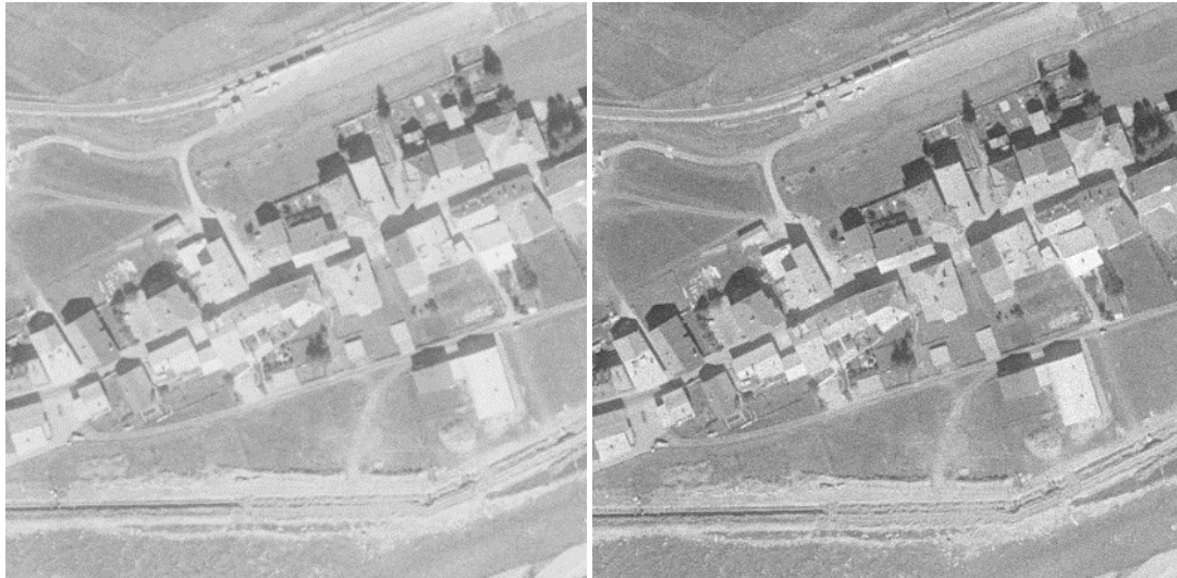
Figure 37: Orthophoto subset before (left) and after (right) the PhotoShop macro. The contrast and the sharpness of the orthoimage is visibly enhanced.
