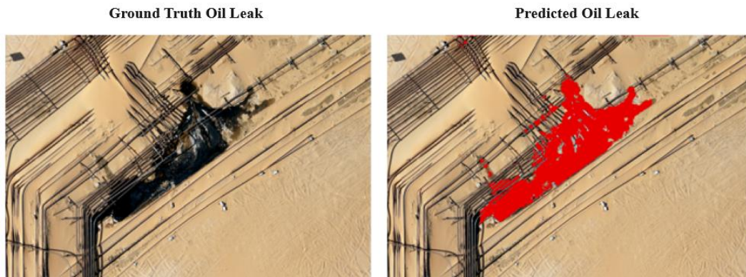
Figure 35. Test Oil Leak Classification Performance of the PSP-Net Classifier
