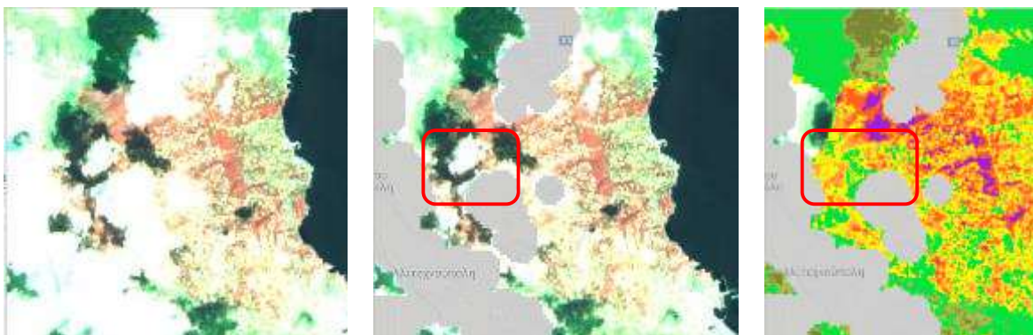
Figure 81: Clouds (left), not detected by the masking algorithm (center) and falsely classified (right).
