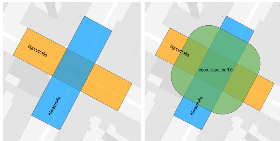
Figure 5.8: Simple intersection and buffer process chain, visualized with QGIS
