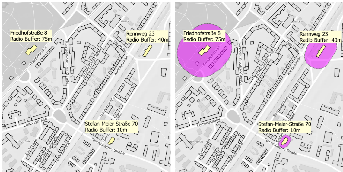
Figure 6.9: Reusability of vect_buffer using the example of building radio systems
