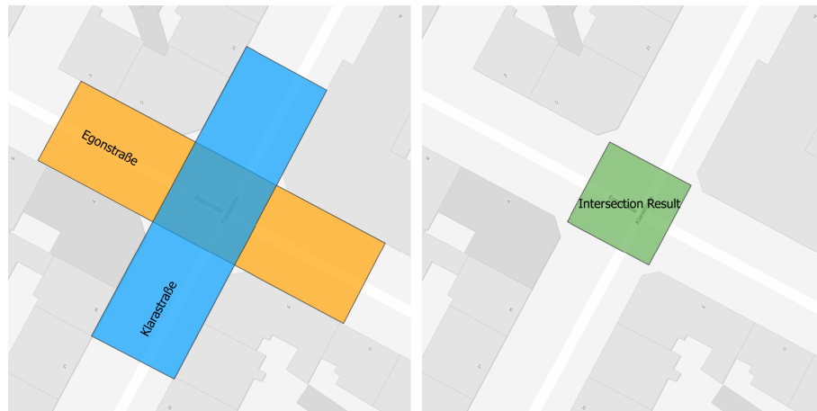
Figure 5.1: Using the intersection process as WPS with two Shapefiles in QGIS
