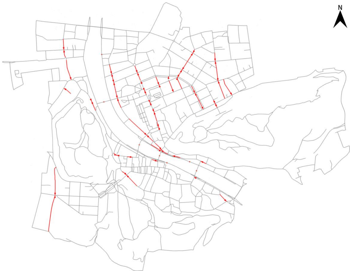
Fig. 2-17: Overview of study area, traffic light scenario 1, cycle 1 (stop roads in red)
