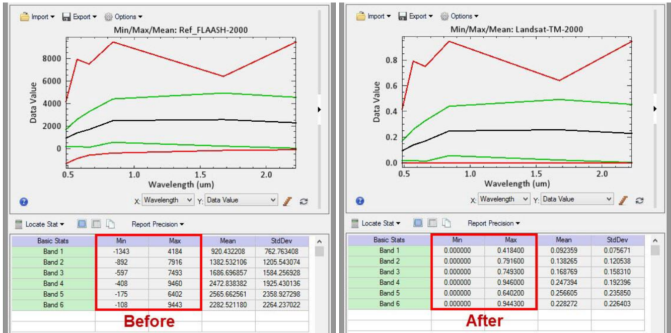
Figure 15: Landsat TM 2000 before and after execution Post FLAASH Band Math Equation.
