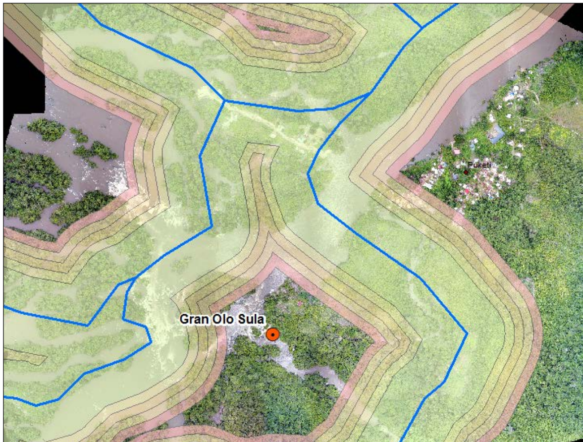
Figure 4-17: Buffers of OSM waterways geometries as a basis for the proximity to water body suitability raster.
