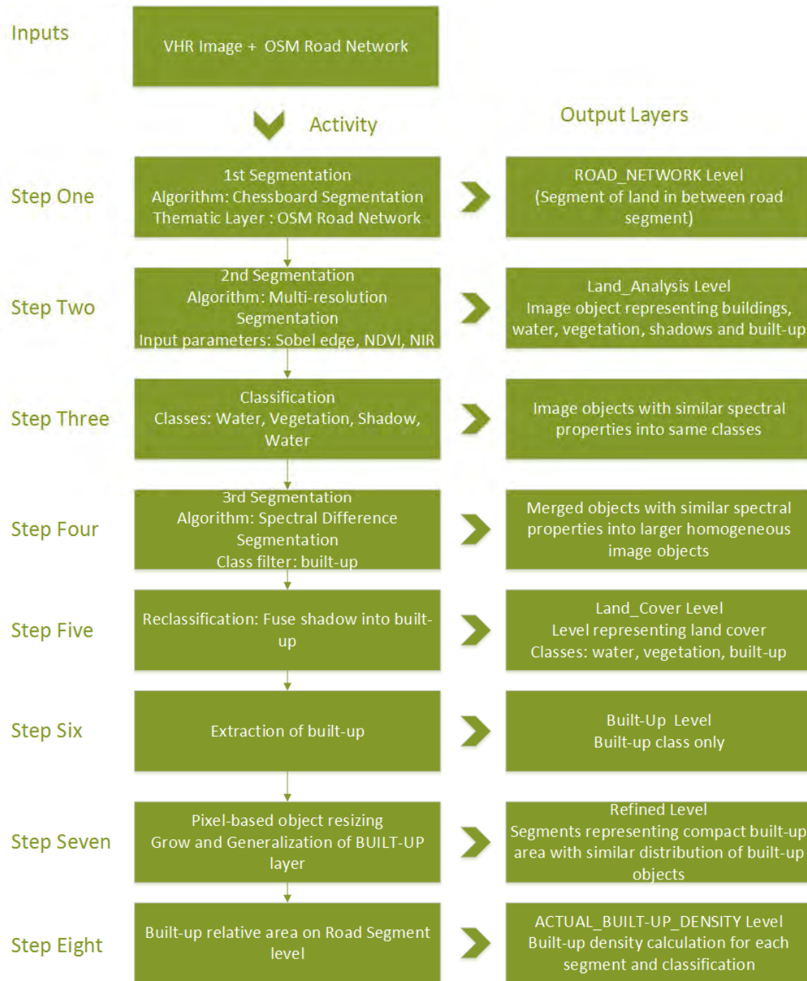
Figure 7 Process flow diagram demonstrating the approach and steps for built-up density classification
