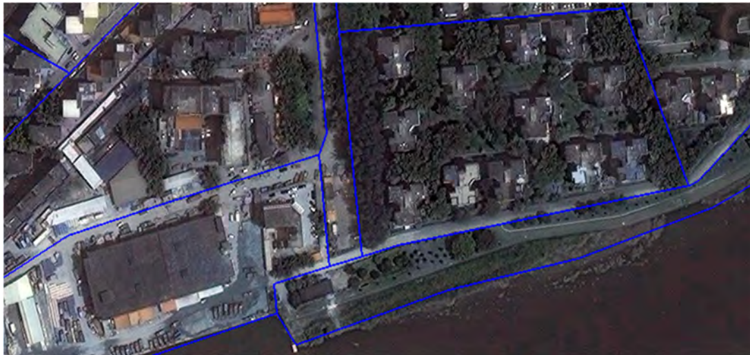
Figure 8 Result of first segmentation - Chessboard segmentation using OpenStreetMap road network on ROAD_NETWORK level
