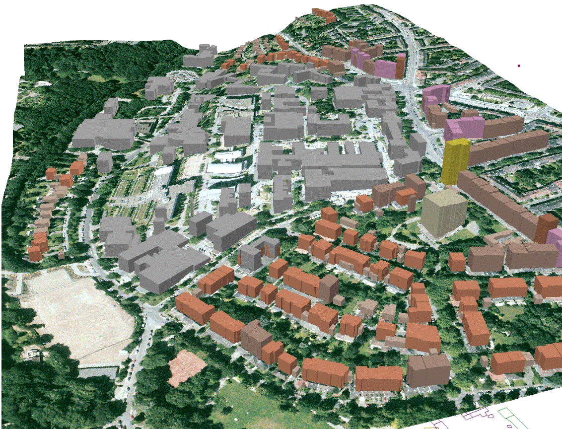
Figure 7.4.2a Animation for a building project in Essen NRW, LoD1 (Virtual Construction support ViCON), CAD Data + 10m grid terrain model + GeoTiff, ArcSecne, Ouput VRML for Navisworks, External Presentation and internal discussion.
