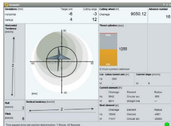
Figure 26: Calculated navigation result on a computer screen (Source: Company VMT GmbH)
