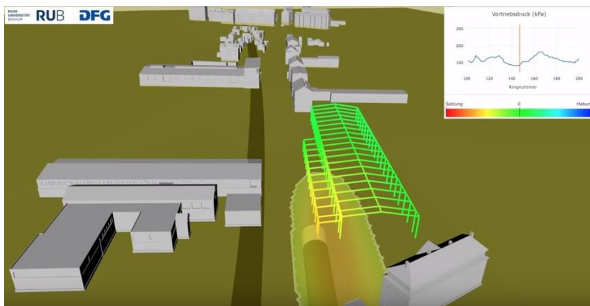
Figure 56: Simulation of TBM advance and effective ground settlements, Source: Bahnprojekt Karlsruhe-Basel, 2016 [online], URL: https://www.youtube.com/watch?v=-L1cJqX7lpE (02.12.2016)
