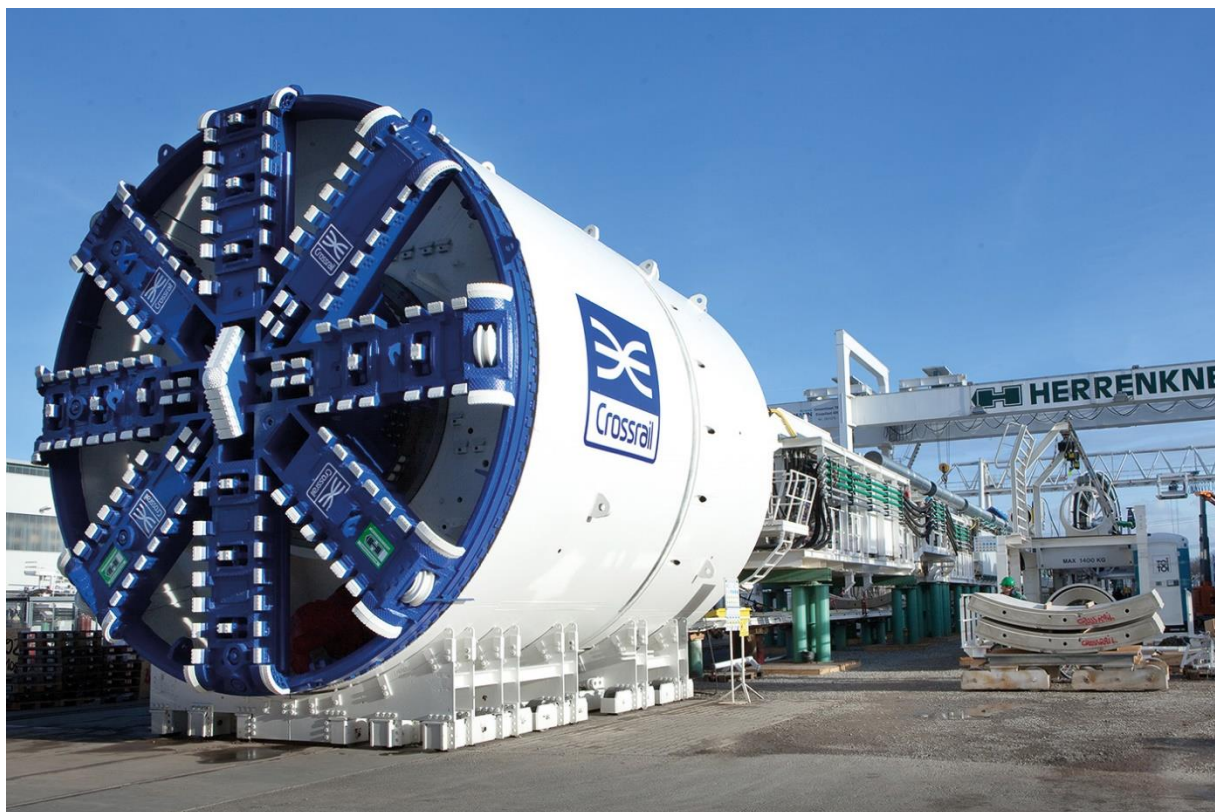
Figure 15: Tunnel Boring Machine in type of an Earth Pressure Balance (EPB) shield for the London Crossrail Project - Source: EPB Machine [ONLINE]. Available at: http://www.Herrenknecht.com [Accessed 16 December 2016].
