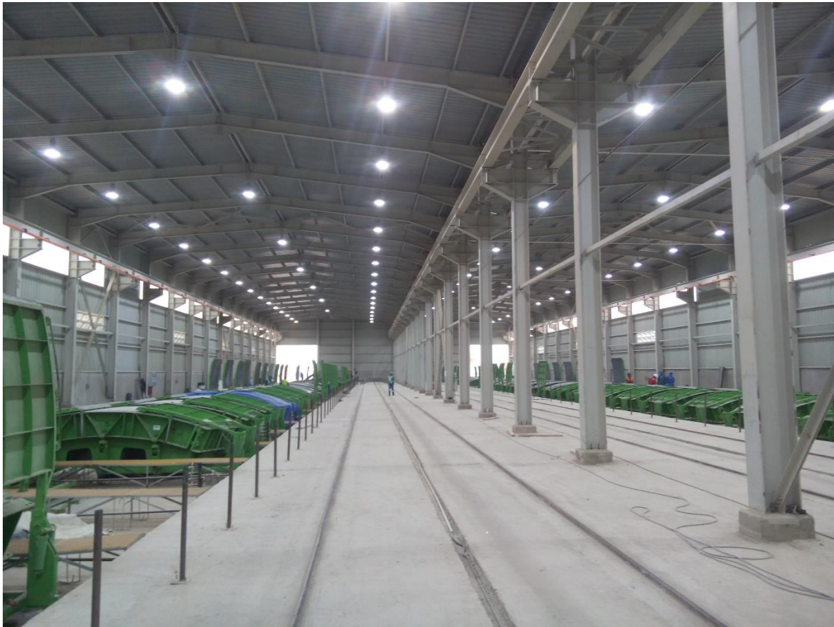
Figure 17: Example of a segment field factory using a stationary production scheme (Source: own imagery)
