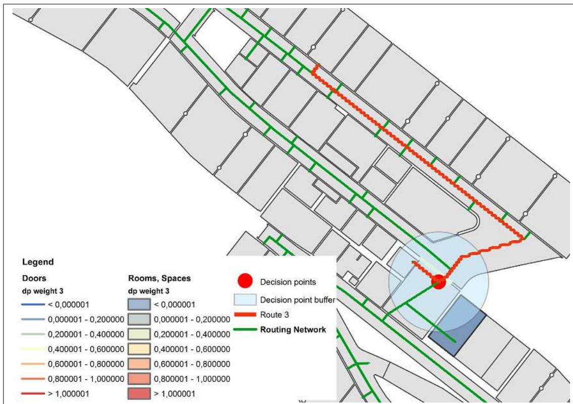
Figure 4.36.: Landmark candidates for decision points of route 3 (third floor) displayed in ArcGIS according to their decision point weight 3
