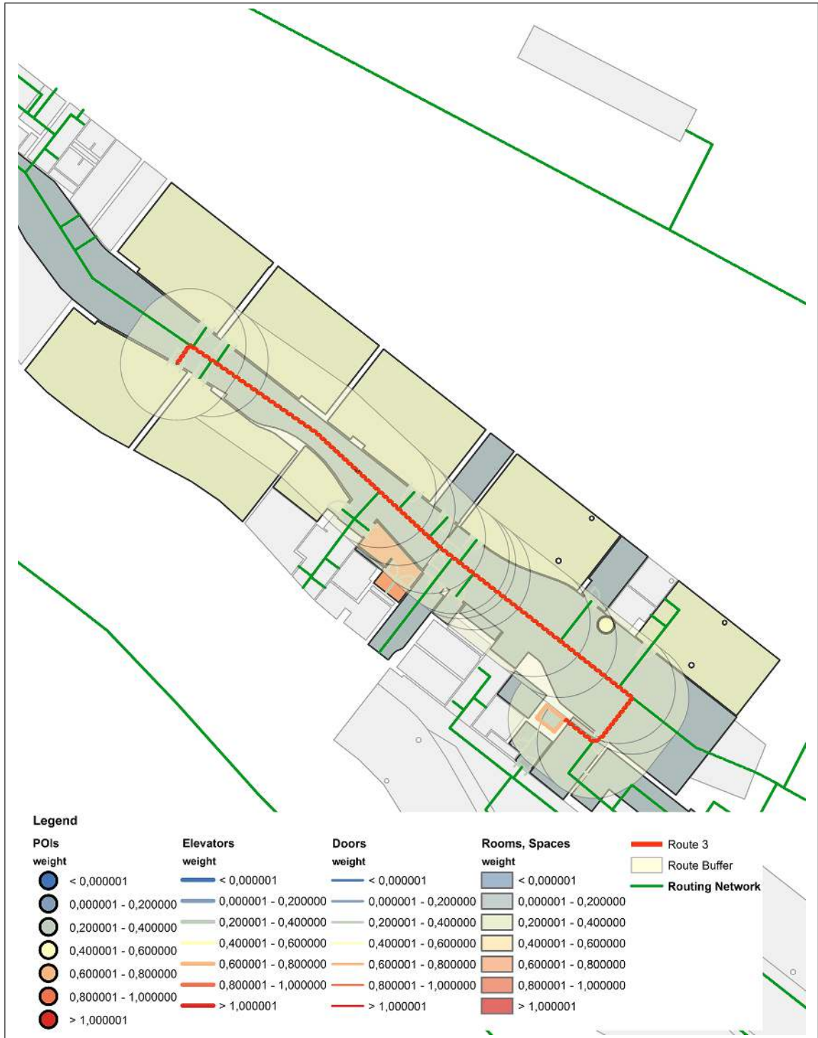
Figure 4.31.: Route 3 (ground floor) with buffer zone and landmark candidates displayed in ArcGIS according to their weight
