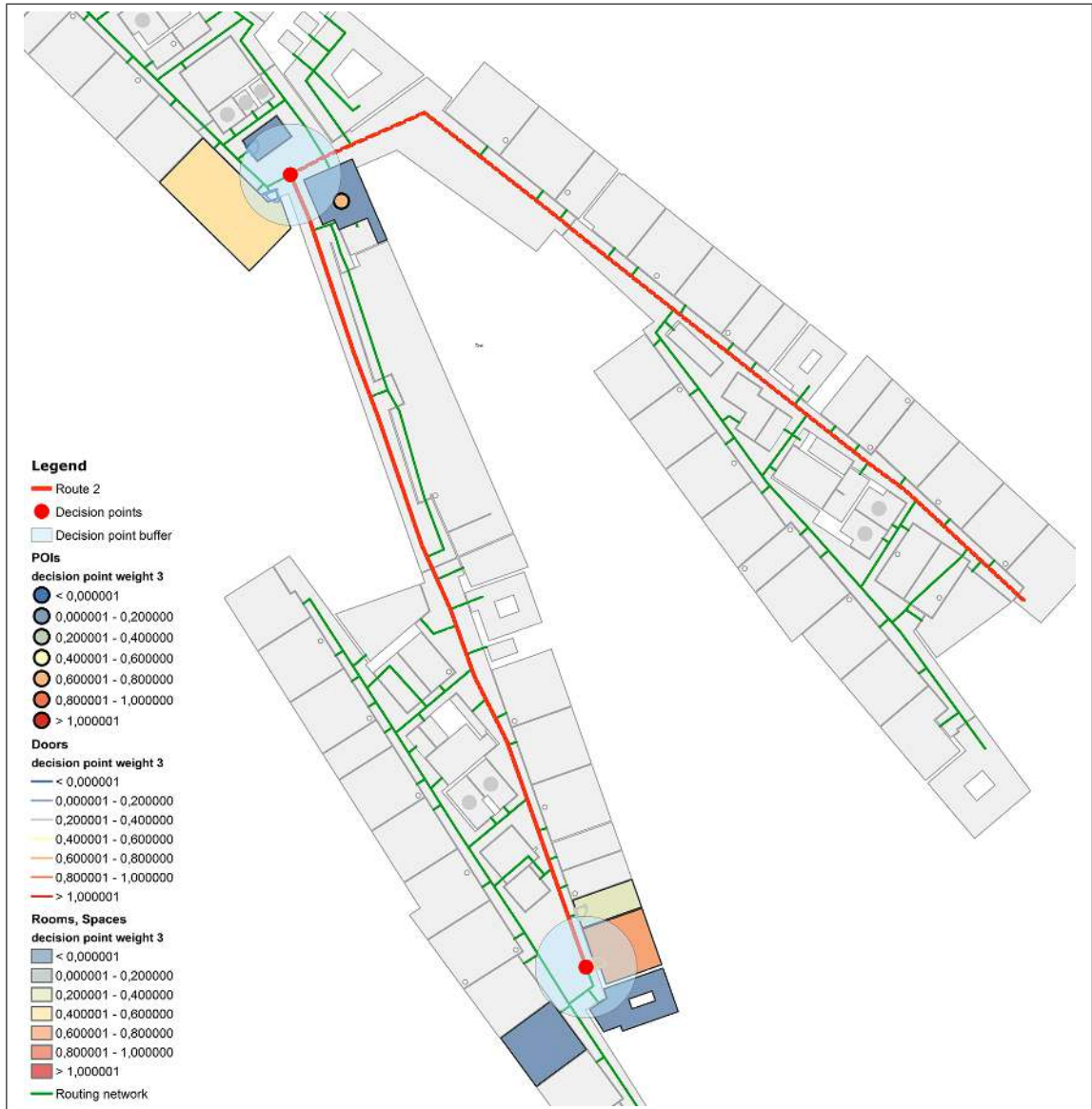
Figure 4.26.: Landmark candidates for decision points in route 2 displayed in ArcGIS according to their decision point weight 3
