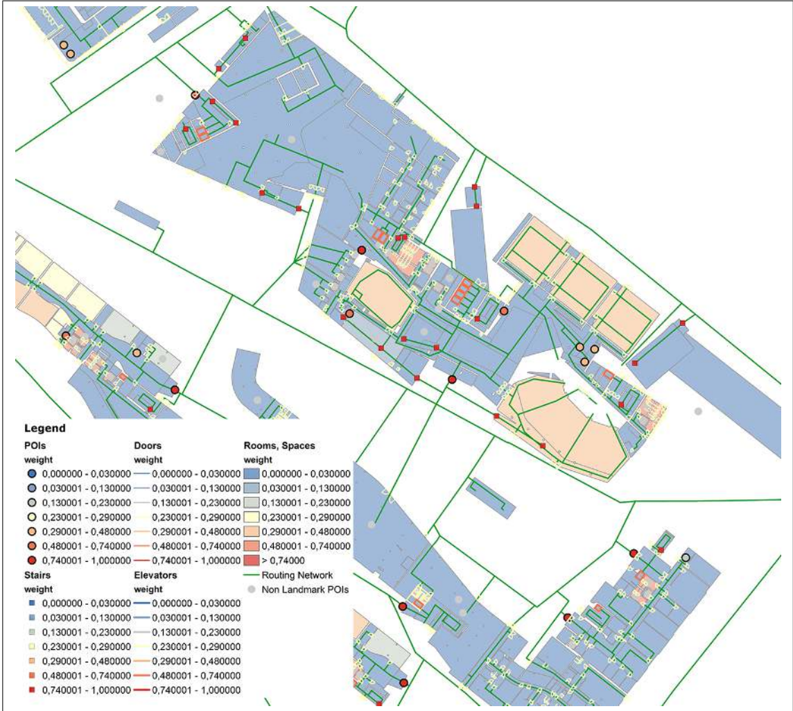
Figure 4.9.: Landmark candidates of the ground floor in Building TC of Campus WU displayed in ArcGIS according to their weight
