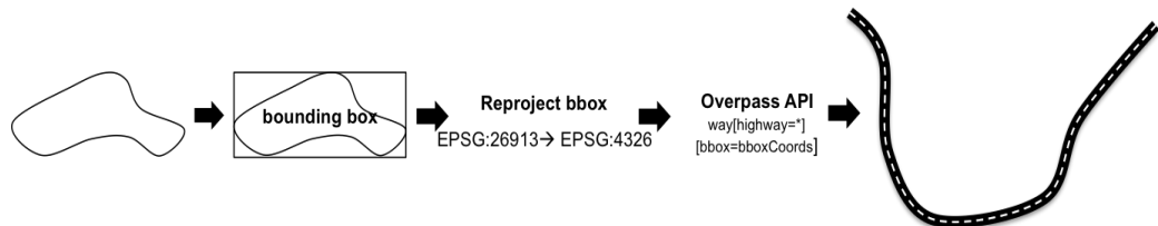
Figure 11: Schema downloadOSMroad function
