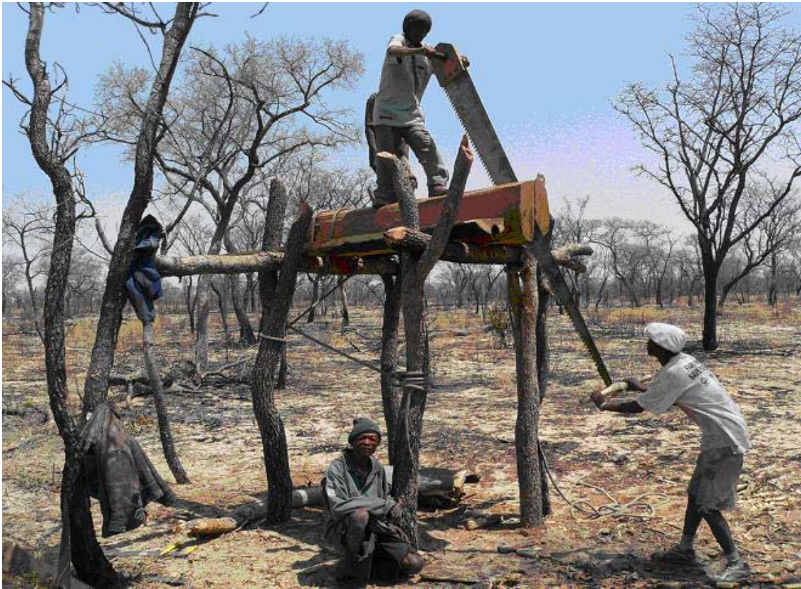
Figure 2. M’Kata community members using long cross-cut saws to produce planks from dead Kiaat trees ( Pterocarpus angolensis ). The current conditional use rights on timber granted by the Department of Forestry (DoF) focus on dead wood utilisation only. A monitoring prototype is currently implemented to determine resource availability in the community forest.
